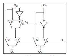
Figure.5 : 2-bit One Adder
