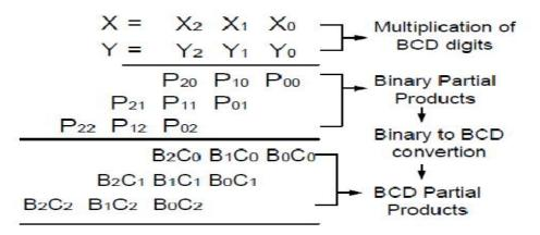
Figure 1: Illustration of BCD conversion in BCD
